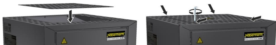
Fig. 19: Installing the cover on model LHT 01/17 D (similar to picture)
