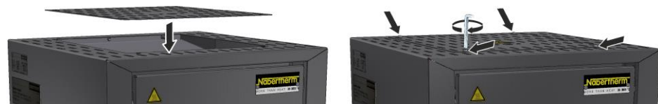
Fig. 51: Installing the cover on model LHT 01/17 D (similar to picture)
