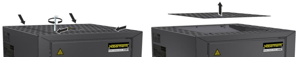
Fig. 17: Removing the cover on model LHT 01/17 D (similar to picture)
