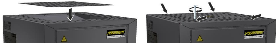
Fig. 39: Installing the cover on model LHT 01/17 D (similar to picture)
